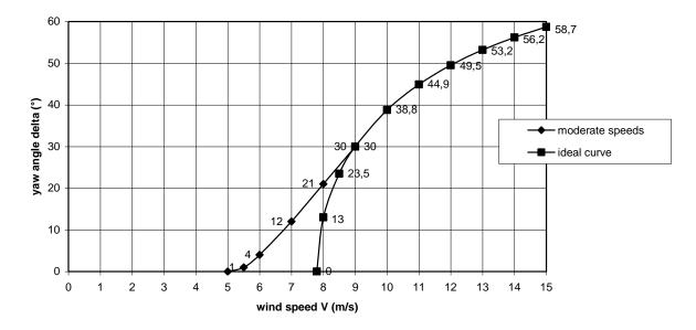
fig. 5 Estimated  $\delta$ -V curve VIRYA-2.2 for a 2 mm aluminium vane blade
