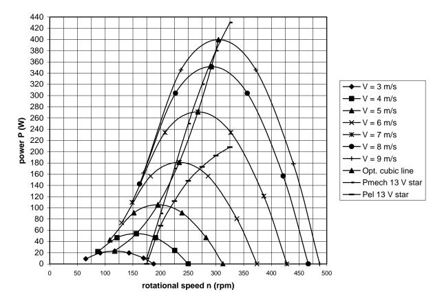
fig. 6 P-n curves of the VIRYA-2.2 rotor, optimum cubic line, estimated P<sub>mech</sub>-n and P<sub>el</sub>-n curves for 12 V battery charging for the chosen winding rectified in star
