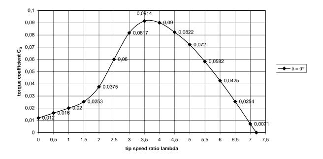
fig. 4 Estimated C<sub>q</sub>- $\lambda$  curve for the VIRYA-2.2 rotor for the wind direction perpendicular to the rotor ( $\delta = 0^{\circ}$ )
