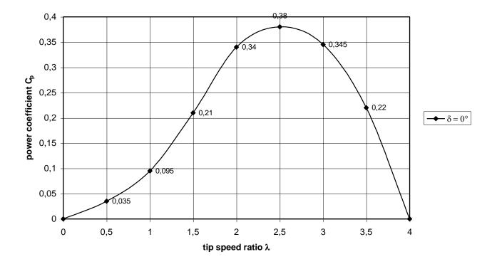
fig. 1 Estimated C<sub>p</sub>- $\lambda$  curve for the VIRYA-2.8B4 rotor for the wind direction perpendicular to the rotor ( $\delta = 0^{\circ}$ )
