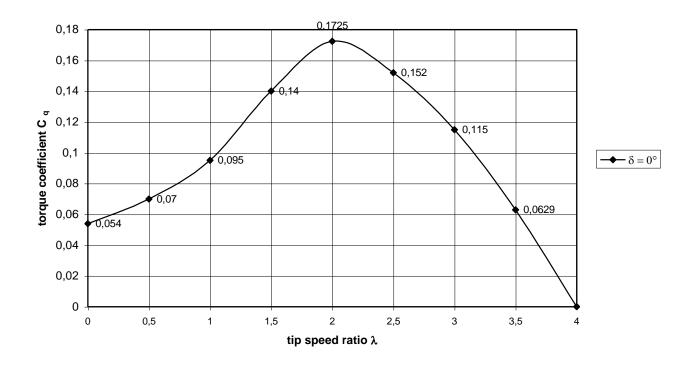
fig. 2 Estimated Cq- $\lambda$  curve for the VIRYA-2.8B4 rotor for the wind direction perpendicular to the rotor ( $\delta = 0^{\circ}$ )
