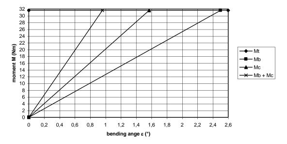
fig. 5 Path of  $M_t$ ,  $M_b$ ,  $M_c$ , and  $M_b + M_c$  as a function of  $\epsilon$
