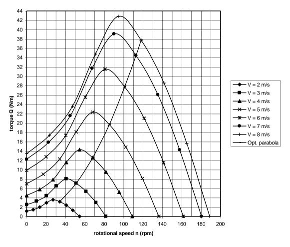
fig. 4 Q-n curves of the VIRYA-2.8B4 rotor
