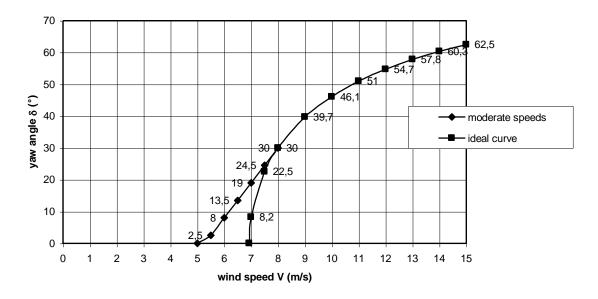
fig. 3 Estimated  $\delta$ -V curve VIRYA-2.8B4 safety system with V<sub>rated</sub> = 8 m/s
