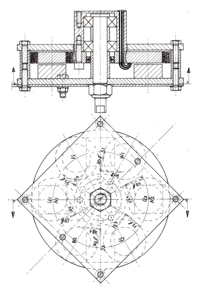
fig. 1 4-pole axial flux permanent magnet generator VIRYA-1.5
