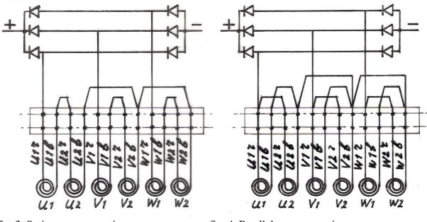
fig. 3 Series-star connection for 24 V battery charging
