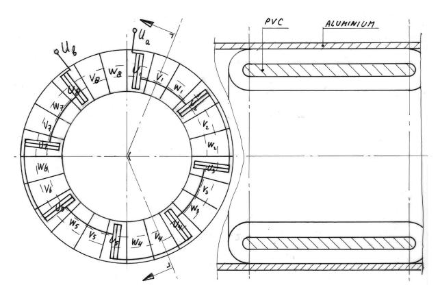
fig. 2 8-pole, 3-phase stator with 24 coils
