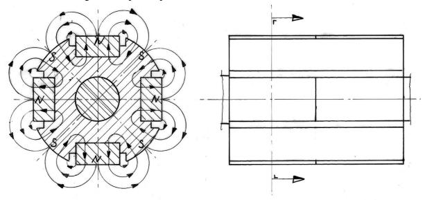
fig. 1 8-pole armature with eight neodymium magnets size 40 \* 20 \* 10 mm.
