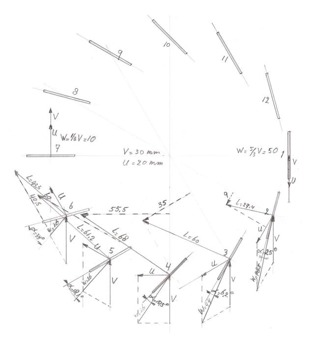
fig. 4 Determination of the tangential components of L for  $\lambda = 2/3$  for positions 2, 3, 4, 5 and 6
